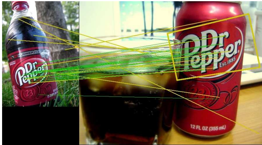
Figure 27 - Dr. Pepper logo matched from Input1 (left) to Input2 (right) using features with counts 0-10 (Input1) and 0-10 (Input2). Matches drawn in green (correct) and yellow (wrong) [12] [13]
