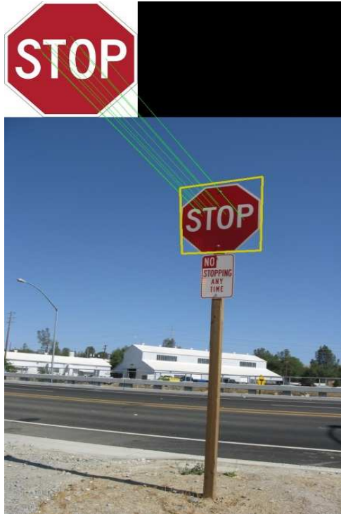
Figure 52 - Stop sign matched from Input1 (top-left) to Input2 (bottom) using features with counts 8-10 (Input1) and count 0-10(Input2). Matches drawn in green (correct) and yellow (wrong) [11] [14]
