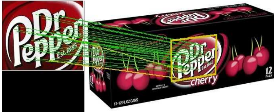
Figure 15 - Brute Force matching result filtered with an orientation angle window [11] [15]
