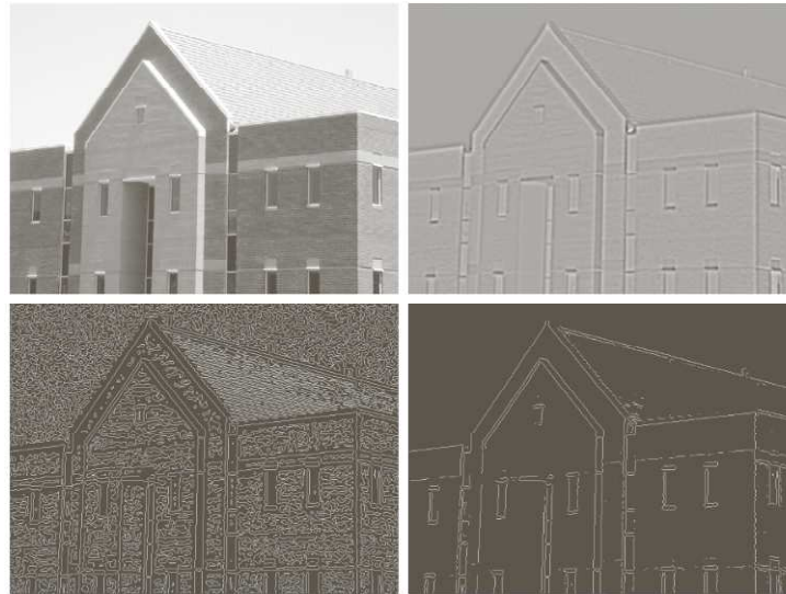
Figure 2 - Top-left: original image, top-right: image convolved with Laplacian operator, bottom-left: zero crossings of Laplacian image, bottom-right: zero crossings with threshold applied [5]
