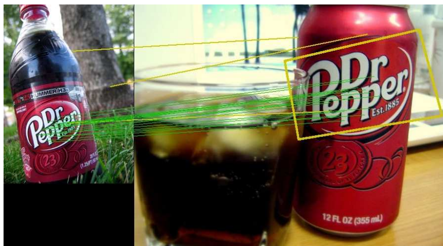
Figure 28 - Dr. Pepper logo matched from Input1 (left) to Input2 (right) using features with counts 6-10 (Input1) and 0-10 (Input2). Matches drawn in green (correct) and yellow (wrong) [12] [13]
