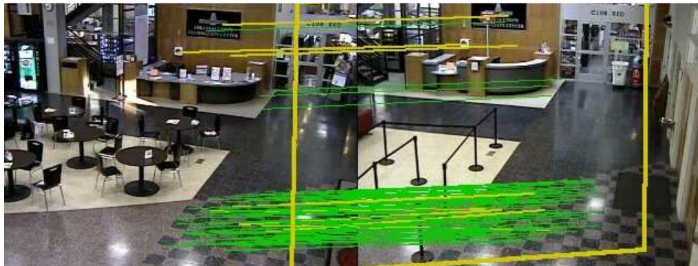
Figure 35 - Input1 (left) to Input2 (right) are matched using features with counts 0-10 (Input1) and 0-10 (Input2). Matches drawn in green (correct) and yellow (wrong) [16]
