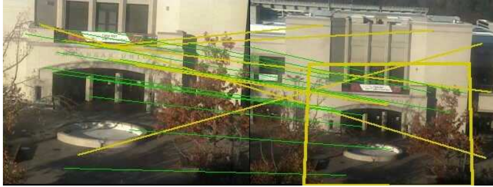
Figure 45 - Input1 (left) and Input2 (right) matched using features with counts 0-5 (Input1) and 0-5 (Input2). Matches drawn in green (correct) and yellow (wrong) [16]
