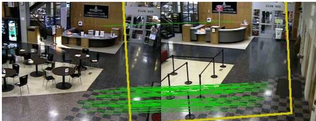
Figure 36 - Input1 (left) and Input2 (right) matched using features with counts 6-10 (Input1) and 6-10 (Input2). Matches drawn in green (correct) and yellow (wrong) [16]
